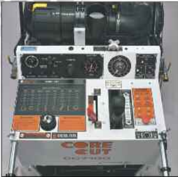
CC7100 Control Panel with drive lever, power raise/lower buttons and gauges
